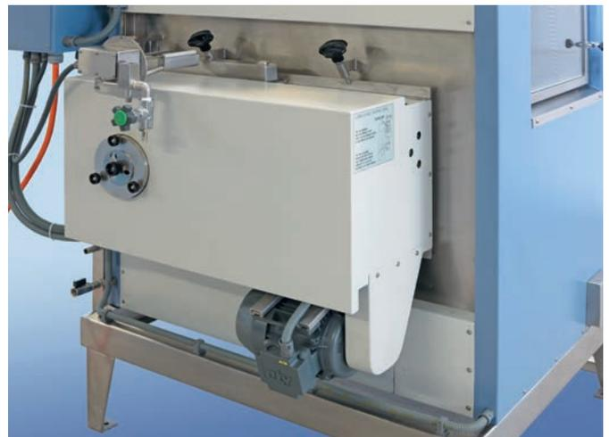
Superheater for temperatures up to 200° C
