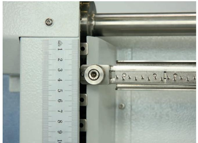
The pin rail can be attached to the transport chain according to the sample
