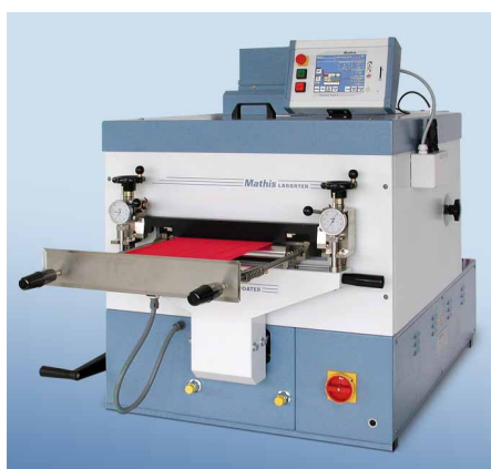
LABCOATER type «LTE-S», the optimum combination of dryer and laboratory coating table. Various kinds of material samples are coated in the same run and heat treated. The coating is applied either by floating, roller or rubber blanket knife. Multiple coatings which do not require re-loading are also possible.
