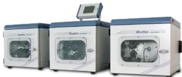
Three LABOMATs «BFA-12» controlled and monitored by one «UNIVISION TOUCH S» process controller
